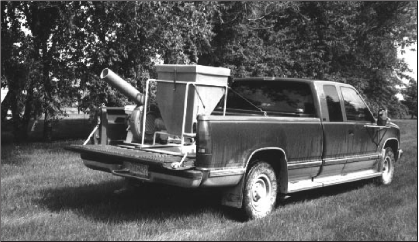
Figure II.19-1 —The Brie-Mar bran spreader fits in the back of a pickup truck and will hold up to 135 lb of bran flakes. This spreader can treat up to a 45-ft swath width. (Photos courtesy of Peacock Industries; used by permission.)
